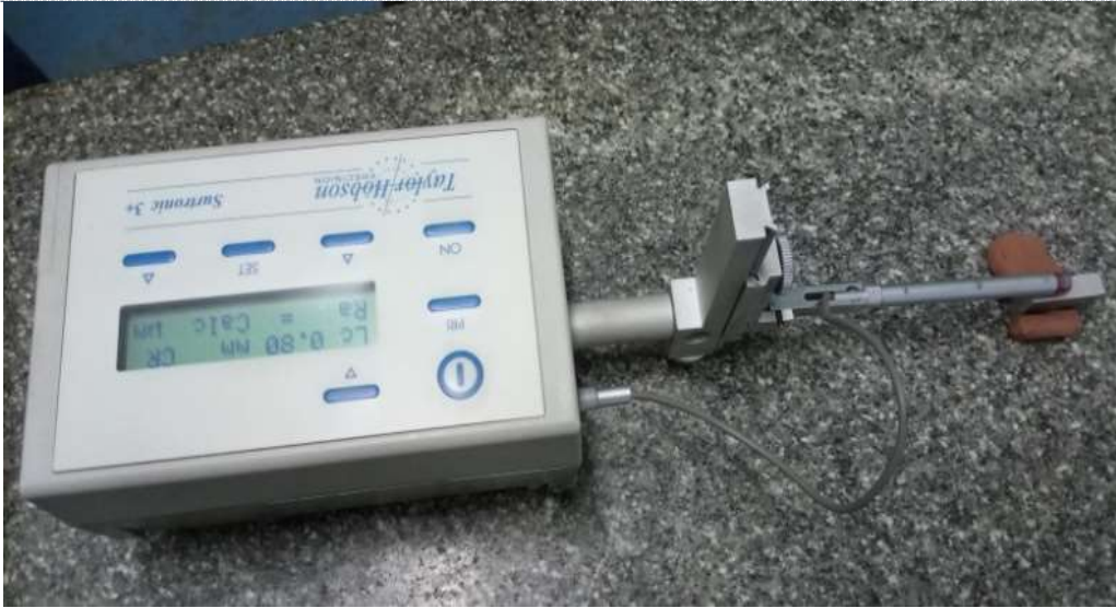
Fig4. Surface Roughness Tester
